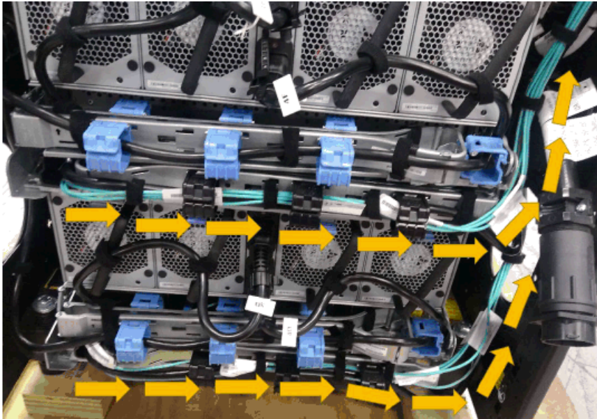
Figure 48. Example of SAS cables routed through the cable management arms
