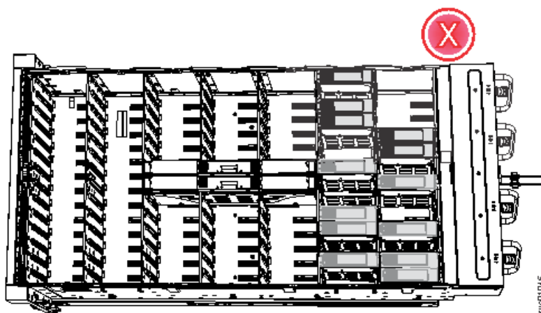
Figure 33. Incorrect drive installation
